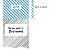
Thick-film passivation approx. 0.4 µm
