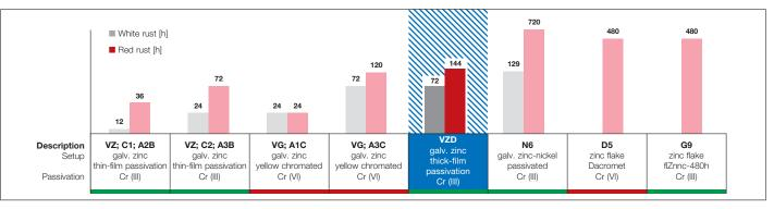
Corrosion resistance of commercially available surfaces, tested in SSN test DIN EN ISO 9227 including description, layer structure and type of passivation shown logarithmically.
