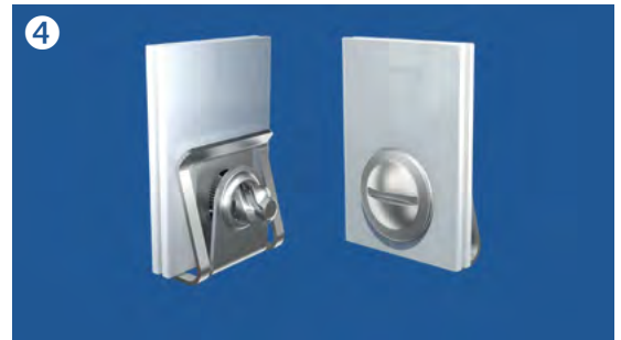
Insertion of the stud into the receptacle. Half a turn is necessary for locking of the joint. Turning it back will release the joint.
